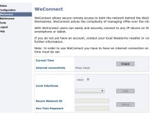
Insert secure network code and OTP to start autoprovisioning
